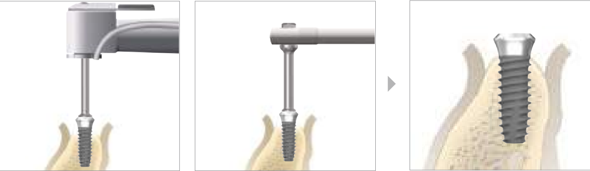
By hand-piece 20rpm / 35N-cm
