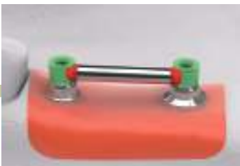
Connect the plastic bar in the middle of trimmed burn-out cylinders to help support the wax pattern. Wax pattern may experience shrinkages.
